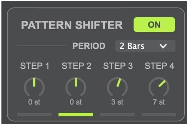
The Pattern Shifter is a built-in 4-step sequencer designed to shift / transpose ACDGEN's main sequence.
